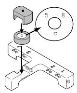
The reference value is engraved on the surface of the supplied reference (such as C 58).
